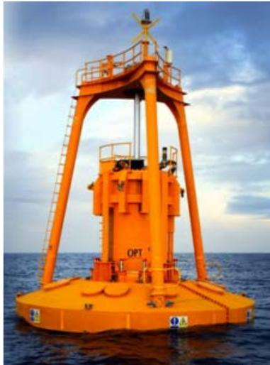
**Figure 2: 150kW rated PowerBuoy deployed off Scotland**
